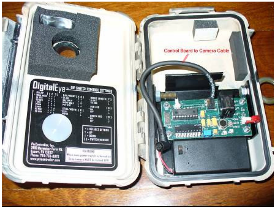
Figure 1: Identification of the Control Board to Camera Cable.
